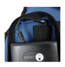
Plug battery back in, controller should beep twice when plugged back into battery
